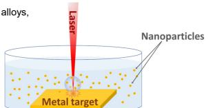
The use of short laser pulses allows to carry out the nanoparticle synthesis process in a wide range of liquid carriers, including volatile organic solvents.
