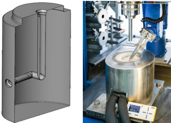
Figure 3: left: Section view through a design drawing of the core of the D-ECAP tool showing the channel with two angles of 90^\circ each. Outside this core, a heating jacket is installed to adjust the desired process temperature. The samples are pressed through the tool by a plunger from the top. Right: Foto of the ECAP tool in the Press.
