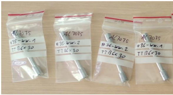
Figure 8: Al alloy samples after ECAP prepared for Tensile testing
