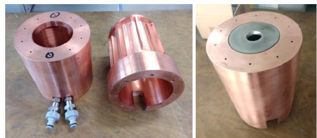
Figure 7: Cooling jacket before soldering; finished cooling jacket with the ECAP die.
